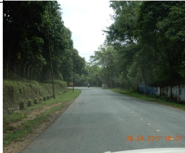
Absence of 'Curve Ahead' Warning Signs and 'Chevron Signs' and trees obstructing the Sight Distance at the horizontal curves between Km. 0/000 to Km. 1/200 on RHS.
