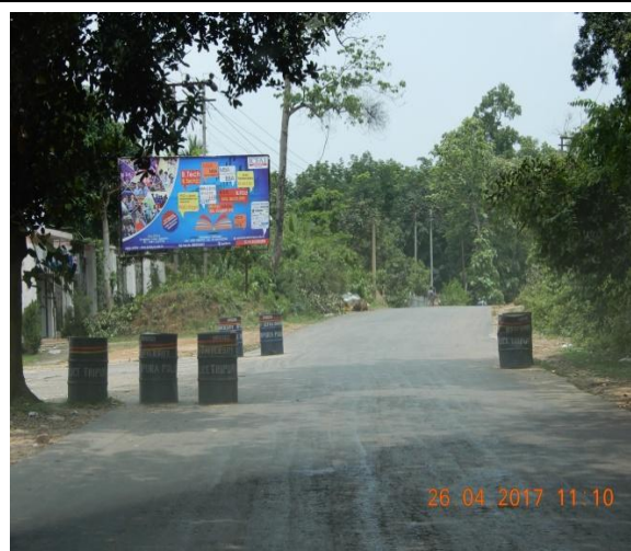
Non-standard Speed Breaker; not conforming to IRC. 67 (2012) between Km 10/000 to Km 13/600.
